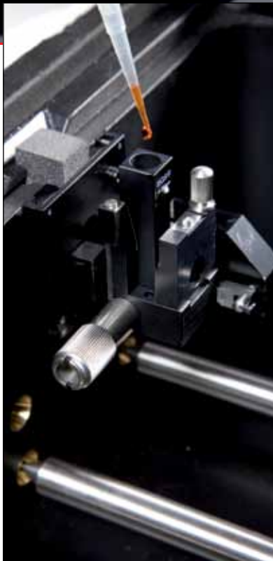
Autosampler for particularly high sample throughput
