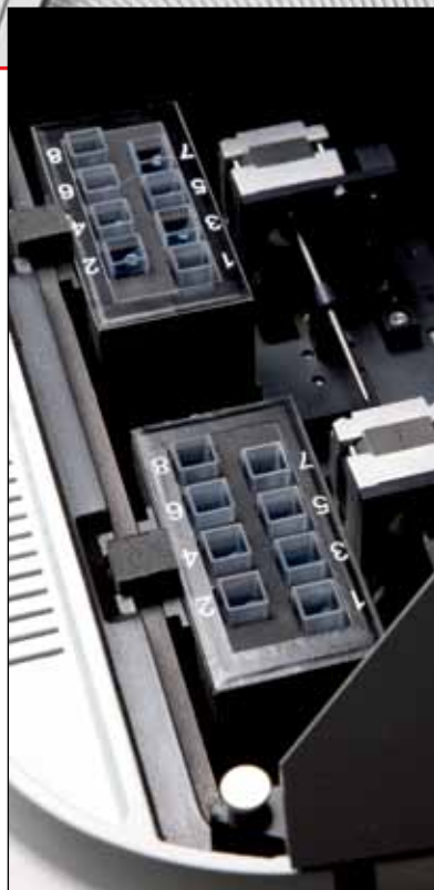
Sipper system for routine quantitative analysis
