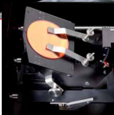
Reflectance attachment with variable angle for determining the refractive index and the film thickness
