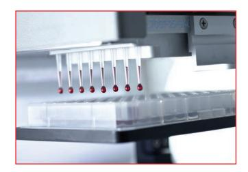
With CyBi®-SELMA you are not restricted to processing only whole microplates. There is an option both in 96-well microplates as well as in 384-well microplates to work column by column. The addition of controls or samples in individual columns, as well as serial dilution is possible at any time.
